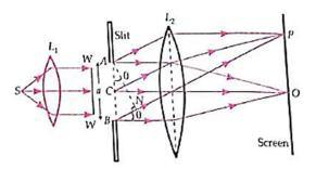
Source S of monochromatic light is placed at the focus of a lens L1 to generate a parallel wavefront WW which is incident on a narrow slit AB of width 'a'. According to Huygens' theory, all parts of this slit becomes a source of secondary wavelets. These spread in all directions, thus causing diffraction. L2 is used as a focusing lens. The screen is places on the focal plane of this lens.
