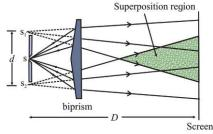
Vertex angle nearly 180°. Very small refracting angle of 30' to 1° with the base. The refracting edge parallel to the slits. The biprism produces  $S_1$  and  $S_2$  as the two virtual sources from the same source S, hence they both are coherent.
